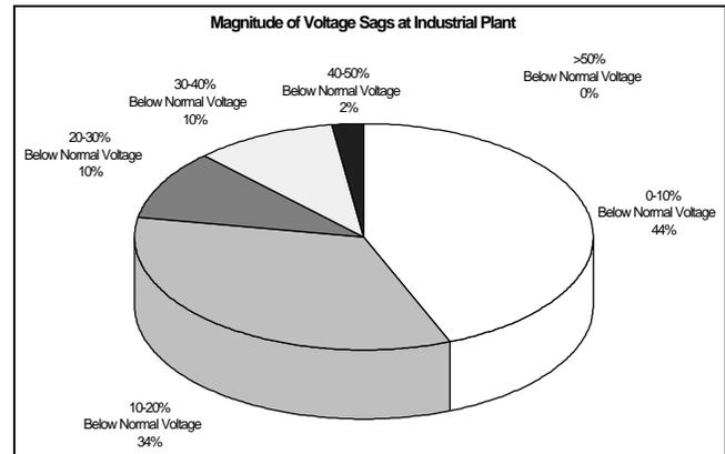
Figure 4. Industrial Plant Sag Magnitude Data (magnitudes are in % below nominal voltage)
