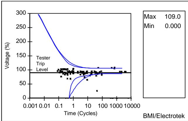
Figure 8. Summary of Voltage Sag Events at Chip Tester Location
