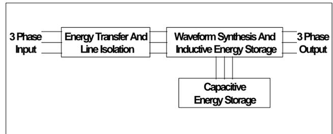
Figure 15. Block Diagram of Magnetic Synthesizer
