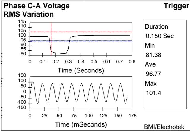
Figure 2. Example Voltage Sag Characteristic During a Fault on a Parallel Feeder Circuit
