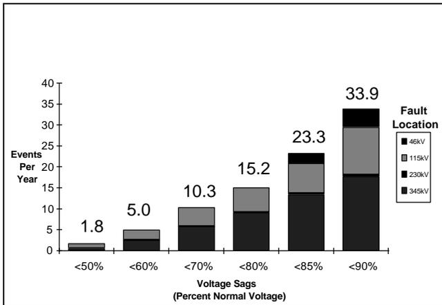
Figure 6. Estimated Voltage Sag Performance at Customer Site as a Function of Faulted Line Voltage and Voltage Sag Level
