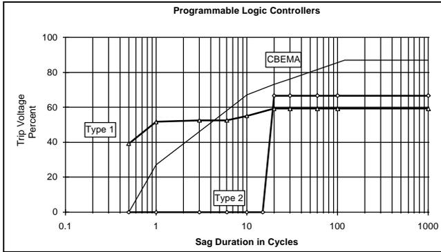
Figure 10. Programmable Logic Controller Ride Through Capability
