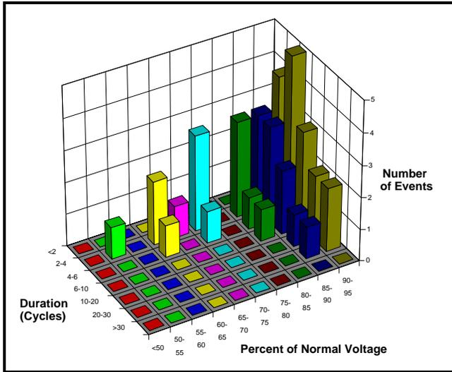
Figure 5. Voltage Sag Events as a Function of Magnitude and Duration
