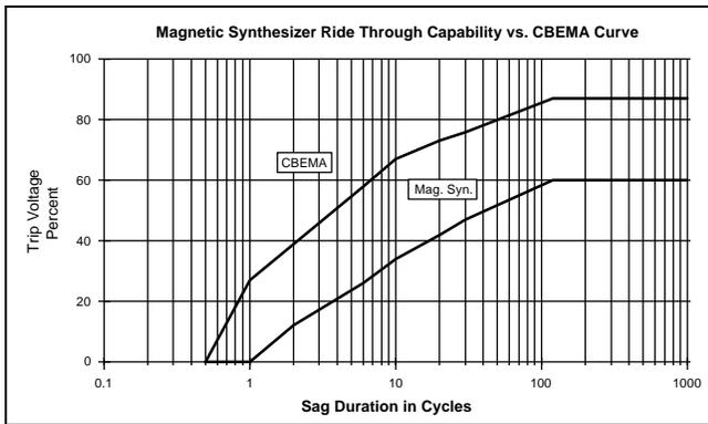
Figure 16. Magnetic Synthesizer Voltage Sag Ride Through Capability
