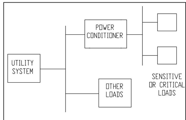
Figure 11. General Approach for the Application of Power Conditioning Equipment
