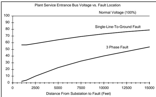
Figure 3. Plant Phase-to-Phase Bus Voltage (%) as a Function of Fault Location on a Parallel Feeder
