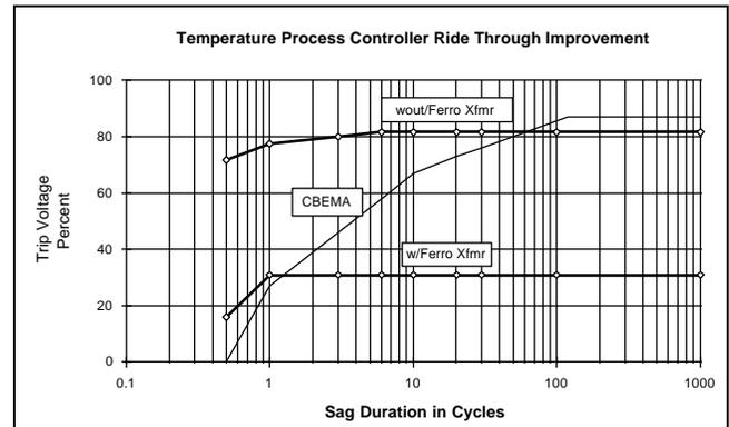
Figure 14. Voltage Sag Improvement with CVT
