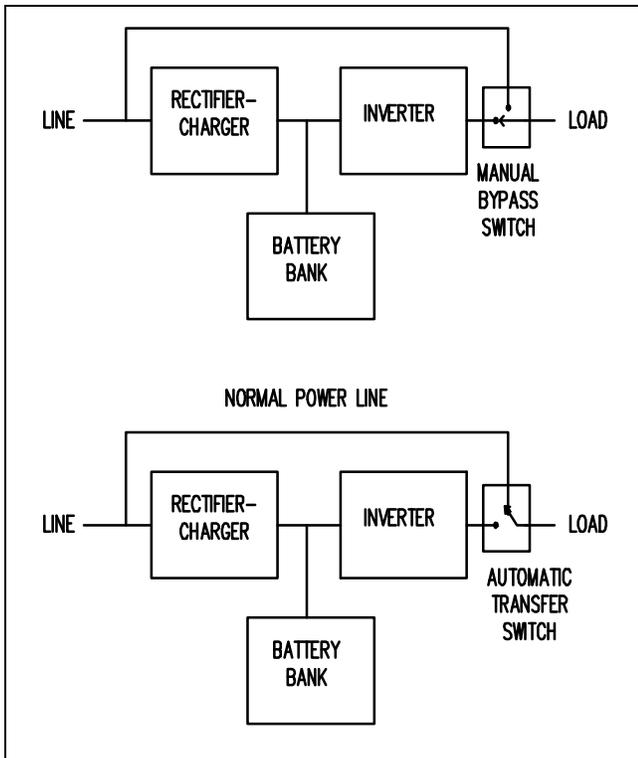
Figure 13. UPS Configurations
