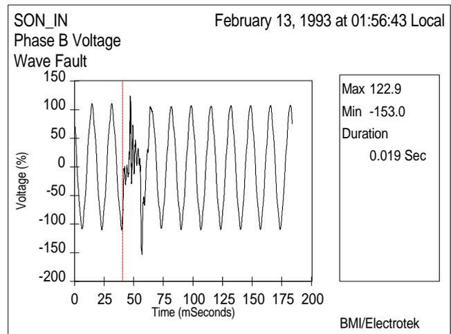
Figure 9. Measured Voltage Sag Disturbance Causing Extruders to Trip
