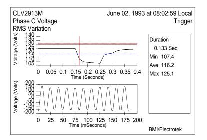
Figure 9. Example voltage sag event with a magnitude of 107V and a duration of 0.133 second.
