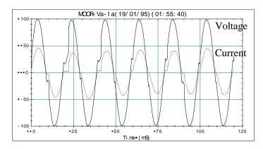
Figure 4. Voltage and current waveshapes from circuit with a loose connection.
