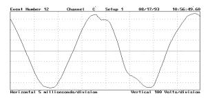
Figure 7. Energization of a capacitor bank as seen from a distance.
