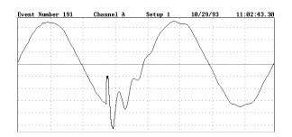
Figure 6. Typical disturbance caused by the energization of a capacitor bank.
