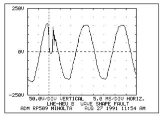
Figure 8. Waveshape fault during the operation of a voltage regulator.
