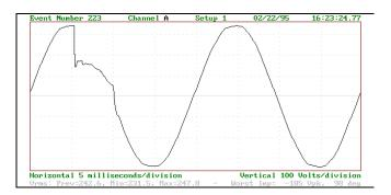
Figure 5. Waveshape accompanying an underground cable failure breakdown.
