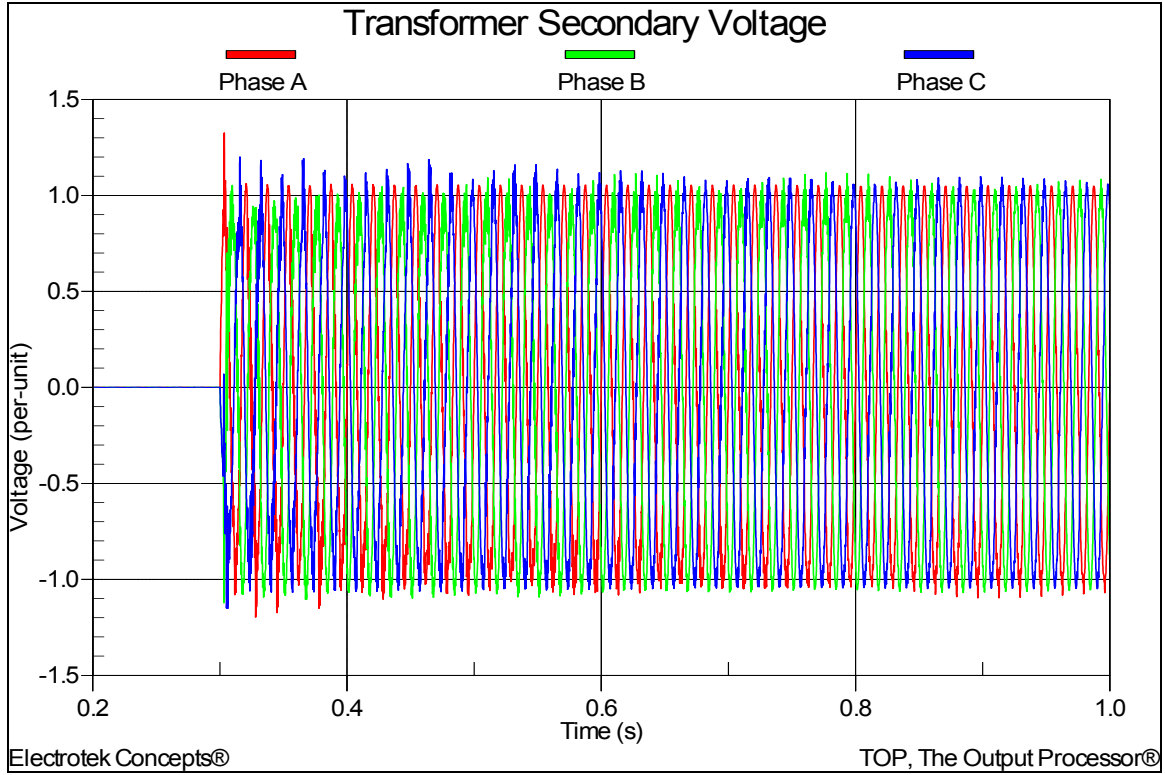
Figure 5 - Simulated Substation Transformer Secondary Voltage for Case 2
