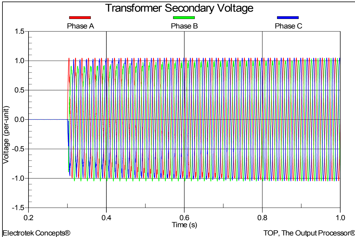
Figure 4 - Simulated Substation Transformer Secondary Voltage for Case 1
