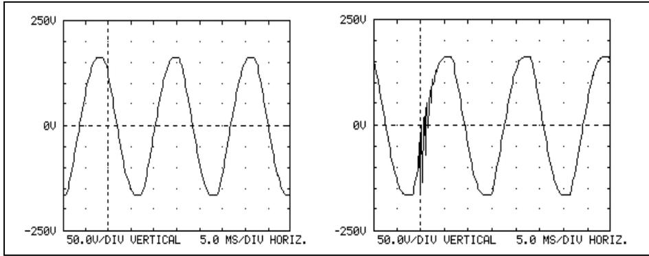
Figure 2 - Low Impedance Power Conditioner Input/Output Waveforms
