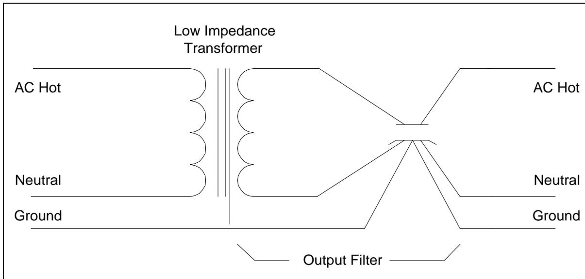
Figure 3 - Schematic of a Low Impedance Power Conditioner
