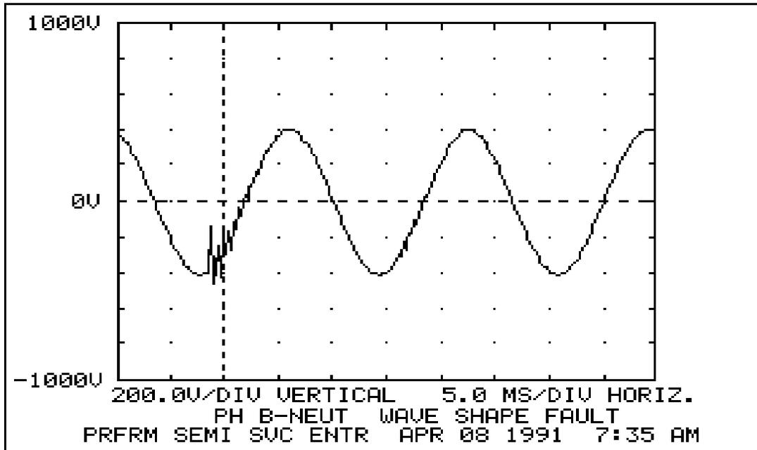
Figure 1 - Capacitor Switching Transient Recorded at the Service Entrance
